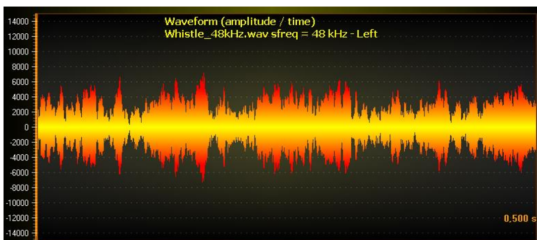
Figure 6-53. Gradient palette coloring for bipolar signal data. UsePalette for Y-axis is disabled.
