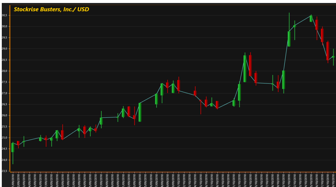
Figure 6-65. StockSeries with CandleStick Style. A light blue PointLineSeries is set to go through all Close values.
