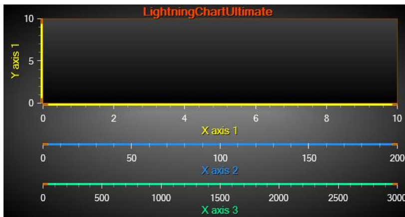
Figure 6-4. XAxisAutoPlacement = AllBottom. Three X axes added, all are positioned below the graph.
