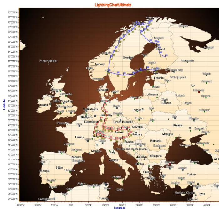
Figure 6-108. Map of Europe, with a couple of FreeformPointLine series as routes. Flag markers are added to them as mouse-interactive waypoints.
