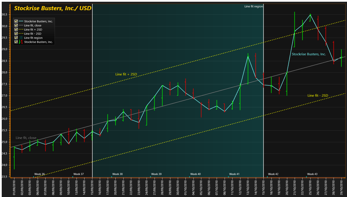
Figure 6-66. StockSeries with Bars Style. Line series are used for showing linear regression fit and offset of that line (2 * standard deviation). A band is used for selecting a date range for line fit.
